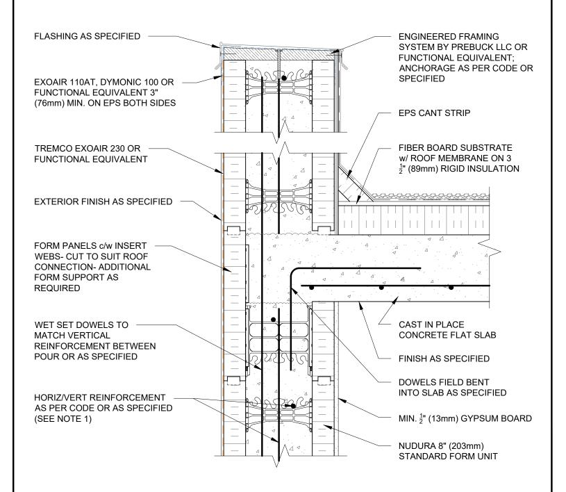
1) FOR OPTIMAL REINFORCEMENT PLACEMENT IN THE NUDURA FORM, SPACING OF HORIZONTAL REINFORCEMENT TO BE SPECIFIED AT 18" (457mm) O.C. AND VERTICAL REINFORCEMENT TO BE SPECIFIED AT MULTIPLES OF 8" (203mm) O.C. REFER TO NUDURA REINFORCEMENT PLACEMENT DETAILS.
