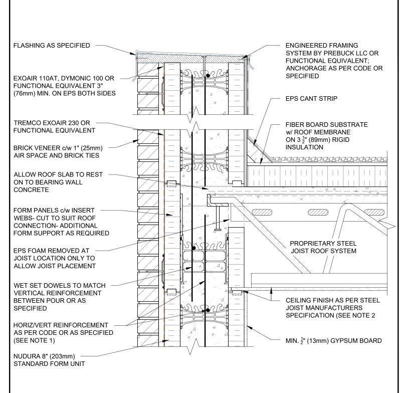
1) FOR OPTIMAL REINFORCEMENT PLACEMENT IN THE NUDURA FORM, SPACING OF HORIZONTAL REINFORCEMENT TO BE SPECIFIED AT 18" (457mm) O.C. AND VERTICAL REINFORCEMENT TO BE SPECIFIED AT MULTIPLES OF 8" (203mm) O.C. REFER TO NUDURA REINFORCEMENT PLACEMENT DETAILS. WHERE GYPSUM BOARD IS REQUIRED TO 2) COMPLETE FIRE RATED ASSEMBLY, EPS FOAM KERF CUT TO ENABLE CEILING FINISH TO PROVIDE THERMAL BARRIER CONTACT TO CONCRETE.
